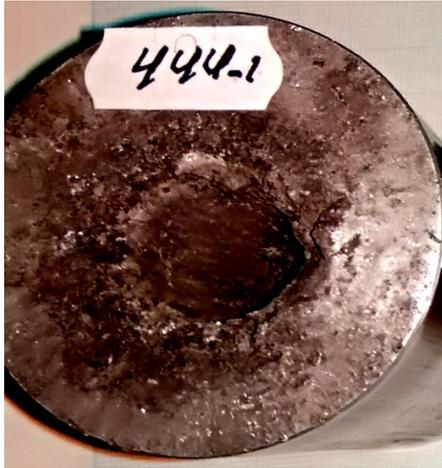
**Fig. 8.** Entrance hole of the cavern (60 mm in diameter) in AMg6 barrier when hit by an aluminum projectile at 10 km/s with a single 3.2 mm “IDEAL” protective screen.
